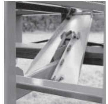
Stainless steel over the top (bandcast) distributor
